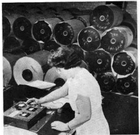
Electrical tests are made during production. Note unfinished stock rolls in background
