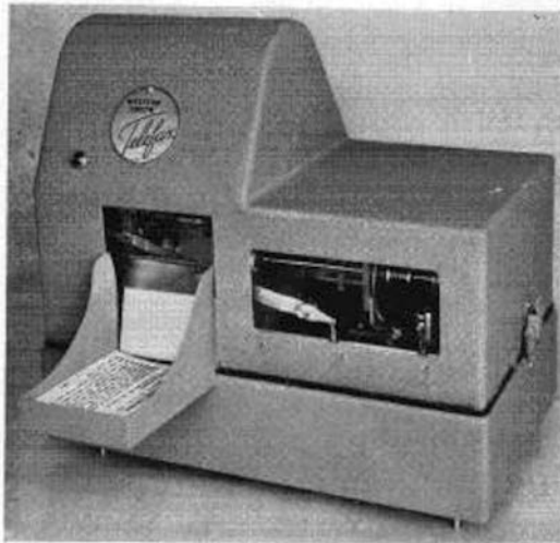
Message-a-minute facsimile telegram recorder used in mobile Telecar motor delivery service
