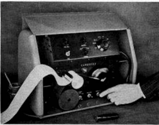
Cardiograph developed in Western Union's research laboratories charts heart impulses
