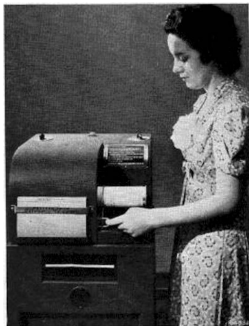
Figure 1. Telefax transmitter-recorder with optical scanning
