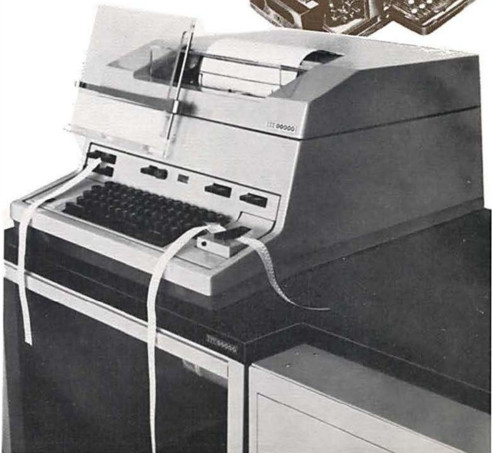
A Model 3 Tape Teleprinter, the first Creed machine produced as a combined start-stop transmitter receiver, in 1927, shadows a Model 444 Teleprinter, the current model in the ITT Creed range.
