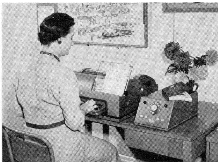
FIG. 13 (b).—TELEPRINTER SET FOR STATION WITH TELEPRINTER ONLY. ON OFFICE TABLE.
