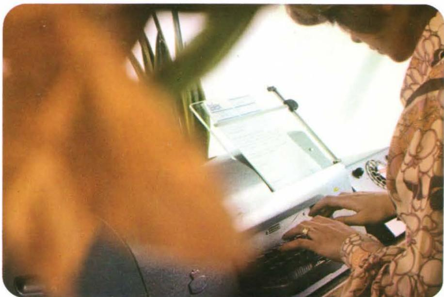
The installation consists of a teleprinter and dialling unit, mounted on a purpose-built table. The teleprinter is similar to an electric typewriter in operation. When a call takes place, identical copies of everything that is typed during the call are printed at both teleprinters.
