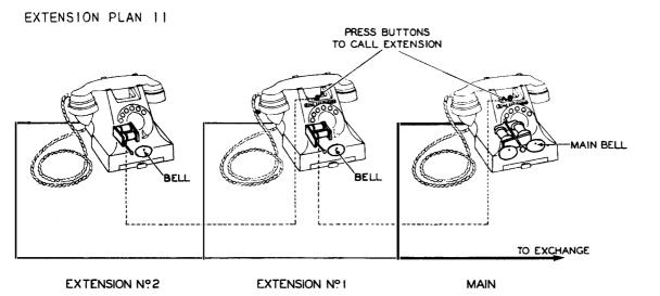
Plan 11. This consists of a main telephone and two internal extensions with 'filtering' facilities. This plan is designed to meet cases where it is desired that incoming calls should be filtered through one extension before being passed on to the other, so avoiding unnecessarily troubling a principal.
