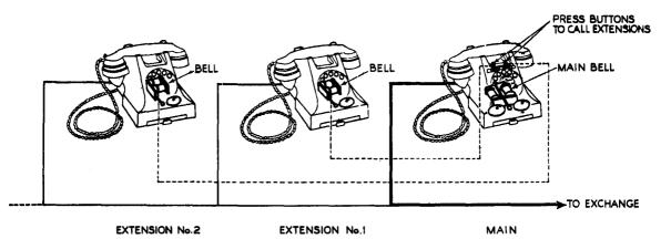
Plan 1A. This consists of a main telephone and one internal extension in parallel. Two extensions may be provided if table telephones are fitted.
