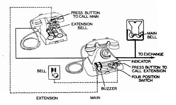
**Plan 7** (internal). This consists of a main telephone and one internal **extension** with intercommunication facilities.
