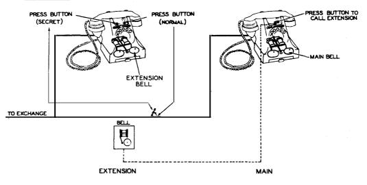
Plan 4 (internal only). This consists of one exchange line with jacks (sockets) in parallel and portable telephone(s), all within the one building. A number of telephone instruments may be supplied; a plug is provided at the end of the cord on each instrument so that it may be moved from jack to jack as required.
