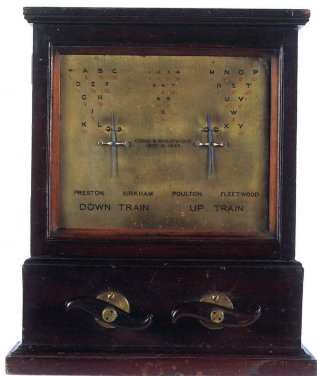
Below: The early needle telegraphs were first used along railway lines - for signalling purposes, as well as to carry messages.
