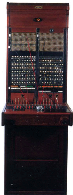
Above: One section from the manual exchange switchboard that used to serve Ossett in Yorkshire until the mid 1960's. A catalogue of designs suited everywhere from the smallest village to the busiest metropolis.
