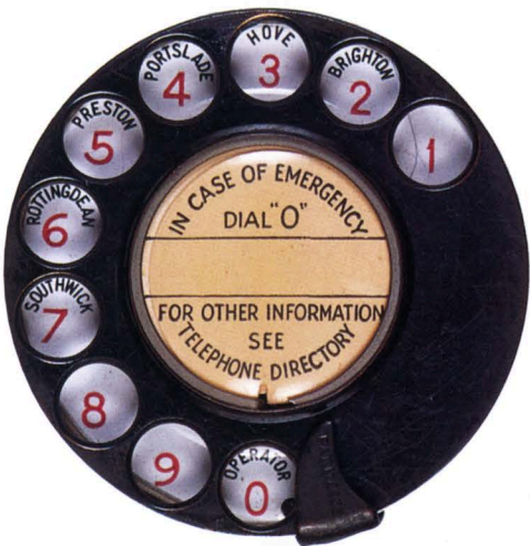
Left: When the Brighton area exchange system went automatic, on 12th November 1927, its subscribers were given unusually helpful dials. Rather than having to remember a range of local codes, callers merely dialled first the name hole and then the number required on that exchange.
