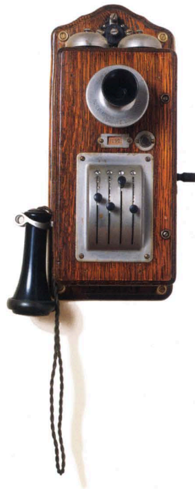
Above: An early Canadian automatic exchange (trialled in Hereford from 1914) used this remarkable 'keyphone' style of telephone. Despite many unique features, the system ultimately proved unreliable.
