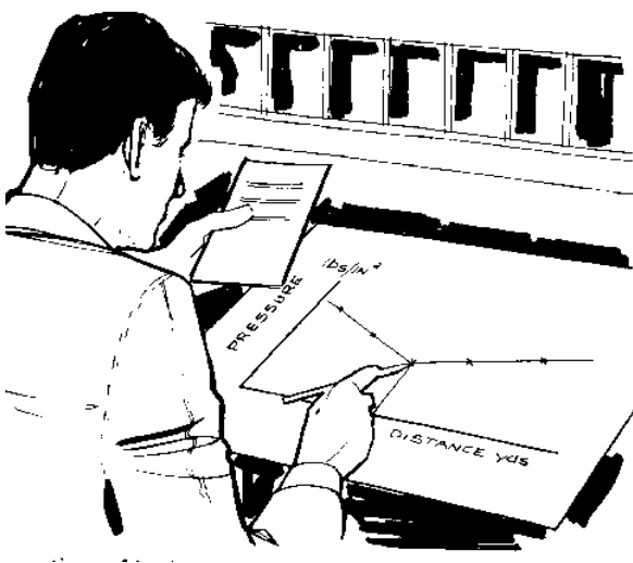
Location of leaks in pressurised cables
