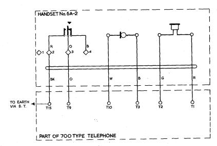
FACILITIES -- CONTROL OF STOP/START FACILITY OF REMOTE DICTATION RECORDING MACHINES BY MEANS OF A PRESS BUTTON LOCATED IN THE HANDSET.
