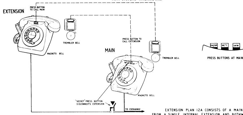
EXTENSION PLAN 12A CONSISTS OF A MAIN TELEPHONE WITH SECRECY FROM A SINGLE INTERNAL EXTENSION AND BOTHWAY SIGNALLING BETWEEN THE MAIN AND EXTENSION. TWO TELEPHONES NORMALLY IN PARALLEL ARE CONNECTED TO ONE EXCHANGE LINE (OR P.B.X. EXTENSION) WITH A SECRECY SWITCH AT THE MAIN,
