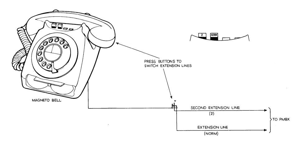
EXTENSION PLAN 9 CONSISTS OF A PRIVATE MANUAL BRANCH EXCHANGE EXTENSION (INTERNAL OR EXTERNAL) WITH A SECOND LINE FOR OUTGOING CALLS. THIS PLAN IS DESIGNED TO MEET THE NEEDS OF AN EXTENSION USER WHO WISHES TO MAKE TELEPHONE ENQUIRIES WHILST HOLDING A PREVIOUS CALL. FACILITIES:-
