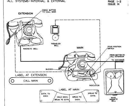
EXTENSION PLANS 7& 7A CONSIST OF A MAIN TELEPHONE WITH A SWITCHING KEY AND ONE EXTENSION (INTERNAL OR EXTERNAL) WITH INTERCOMMUNICATION.
