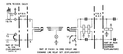
CIRCUIT OPERATION ON EXTN. TO EXCH. CALLS When the button is pressed the earthed loop condition holds the main exchange equipment and operates the differentially connected relay D. Contact D1 lights the supervisory lamps. On extension to extension calls the operator is recalled by using the receiver rest.
