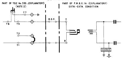
CIRCUIT OPERATION ON EXTN. CALLS. Depression of recall button releases supervisory relay and lights supervisory lamps.
