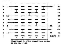
BATTERY SUPPLY VIA FUSE NO.35/1, ONE PER FOUR CIRCUITS. WHEN SIGNALLING CURRENT, MEASURED BETWEEN TAGS 49 AND 50, IS LESS THAN 8 MA.OMIT STRAP BETWEEN 49 AND 50, AND INSERT ADDITIONAL CELLS COMMON TO ALL UNITS IN SERIES BETWEEN NORMAL BATTERY SUPPLY AND TAG 49. SIGNALLING VOLTAGE NOT TO BE INCREASED TO SIGNAL OVER FAULT NOR TO EXCEED 50 V.
