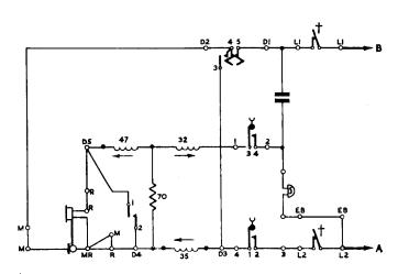
$\dagger$  isolating switch contacts. Break when inner door is opened.
