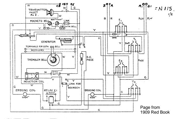
Telephone No. 15. The description includes Cord, Flexible, No. 222; Coil, Induction,  $\frac{25}{1}$ ; Switch; Relay, E<sub>1</sub>, 4,000 ohms; Transmitter, Inset; Generator, Bracket, 3-terminal, unmounted; Condenser, m.c., 1 m.f.; Receiver, Bell; and 4 fixing screws and washers.
