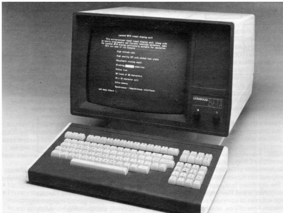
The Lynwood BETA Visual Display Terminal – typical of the equipment now being maintained and repaired by BT.
