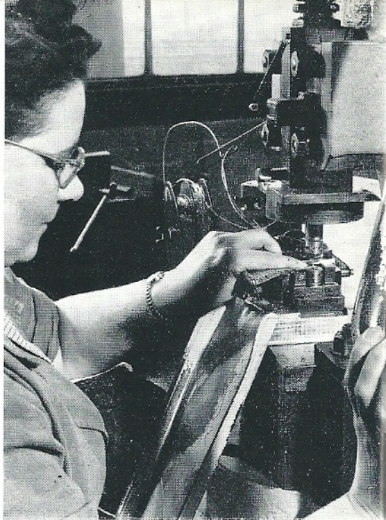
Fitting contacts into relay springs
