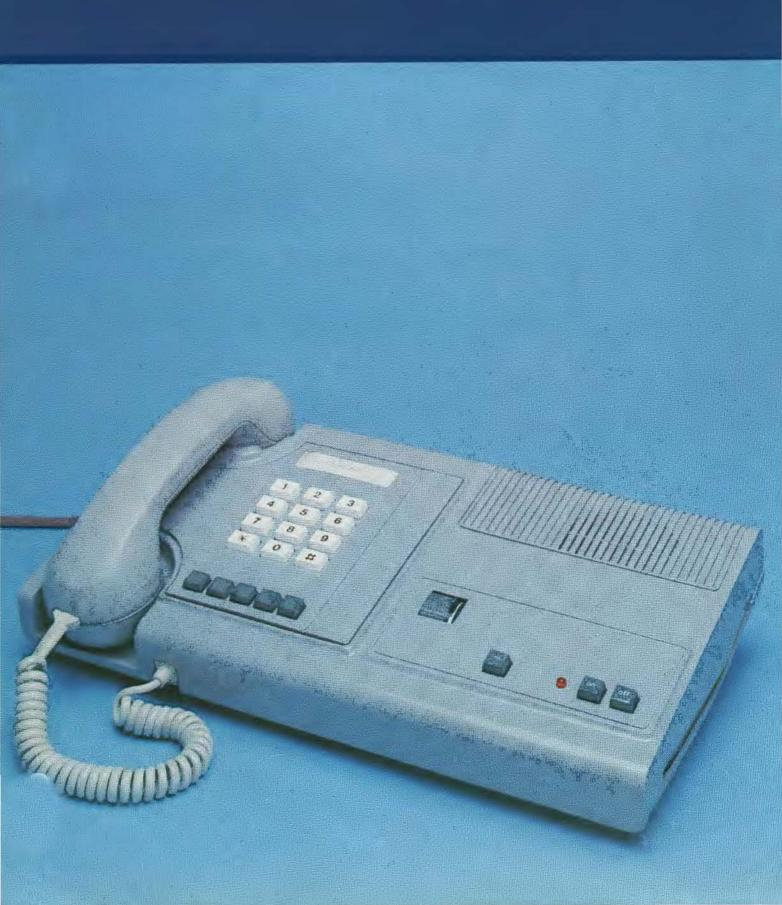
HARMONY LOUDSPEAKING UNIT Harmony can be associated with any telephone to 'convert' it into a loudspeaking telephone.
