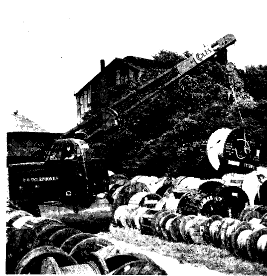
A self-mobile crane
