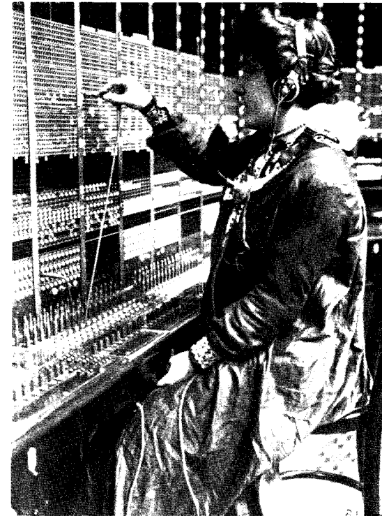
Fig. 3: A typical telephonist about 1900 wearing a type of head-gear receiver and breast-plate transmitter very similar to the present standard operating instrument
