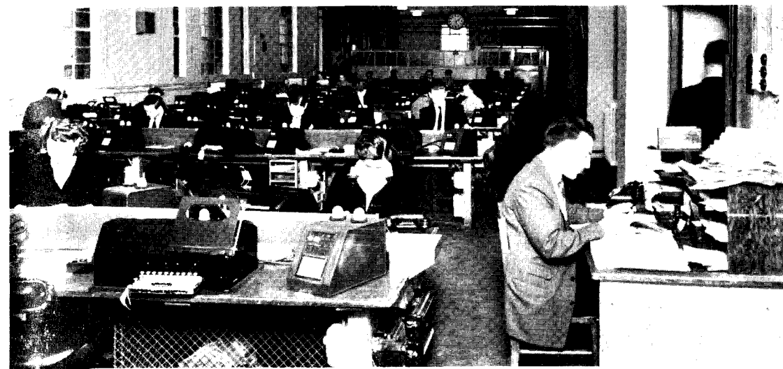
New suite of printergram positions in Central Telegraph Office, London, which serve the new telex system; all telegrams to and from subscribers in London and the Home Counties are handled here
