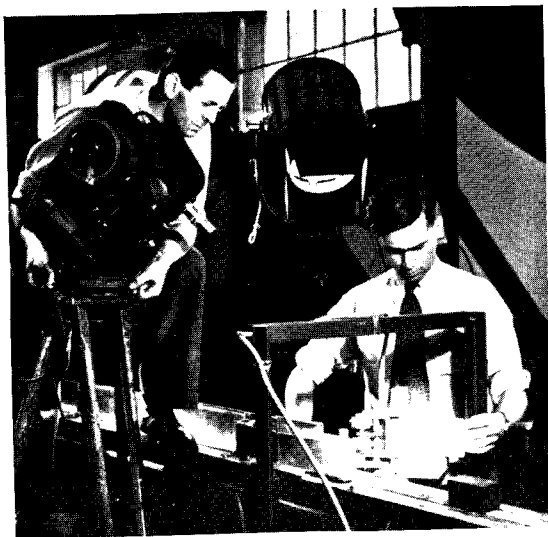
Fig. 4 Taking a high-speed cine film of a mail-handling device
