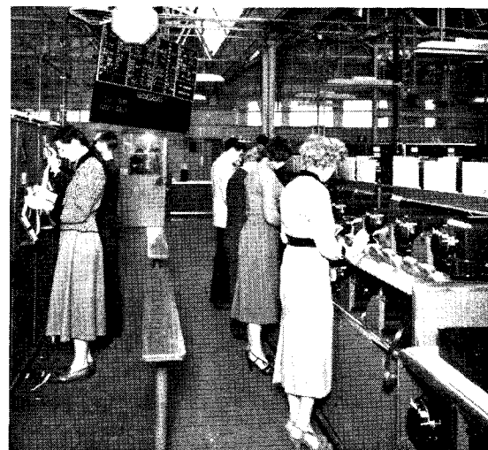
Figure 4: Printing reperforator cabinets (left) and automatic transmitters (right)
