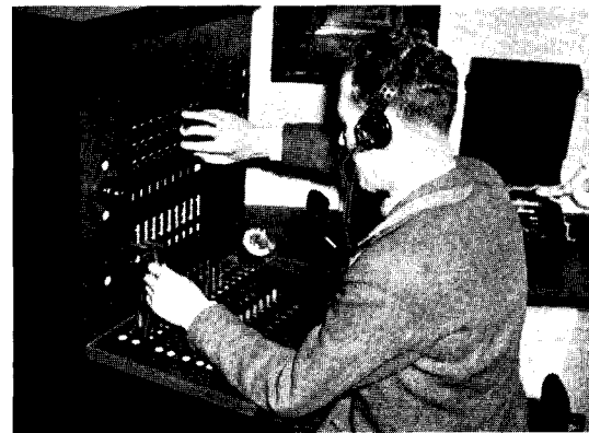
Fig. 2. Identifying the calling indicator by touch. (This learner, Mr. J. Lewis, now operates a Government Laboratory P.B.X.)—Associated Press photo.
