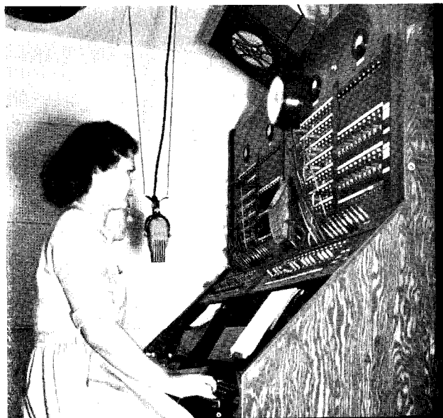
FIG. 7. TELEPRINTER SWITCHBOARD, SHOWING MICROPHONE AND LOUDSPEAKER
