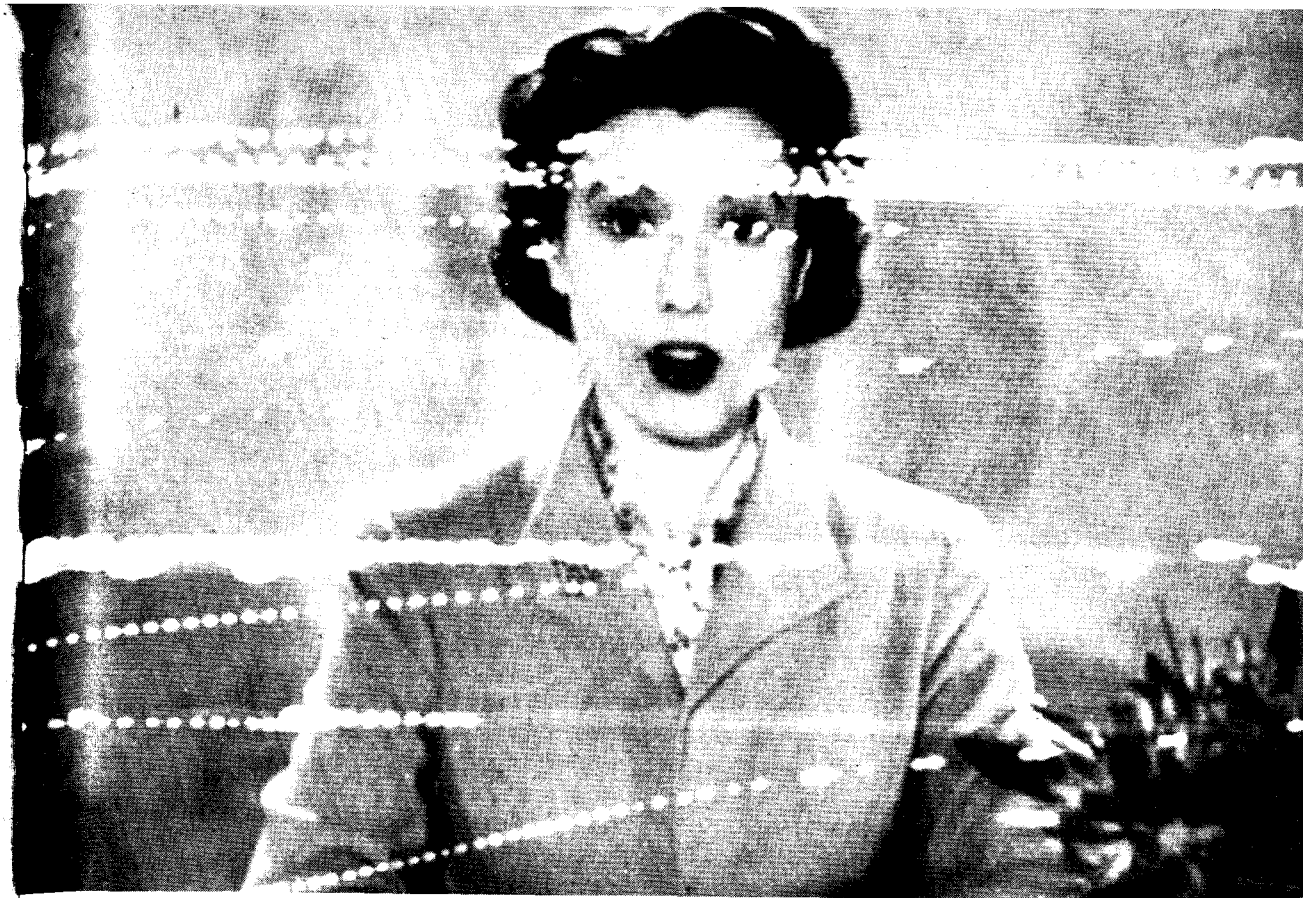
FIG. 2—IGNITION INTERFERENCE WITH TELEVISION RECEPTION.
