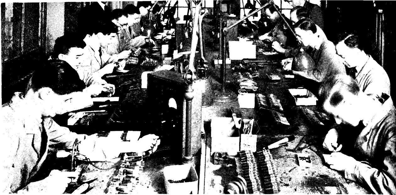
Relay assembly adjustment and testing in progress at London Piece Part Depot
