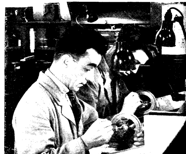
Fig. 8. The Relay Shop. The staff are adjusting 3,000-type telephone relays.
