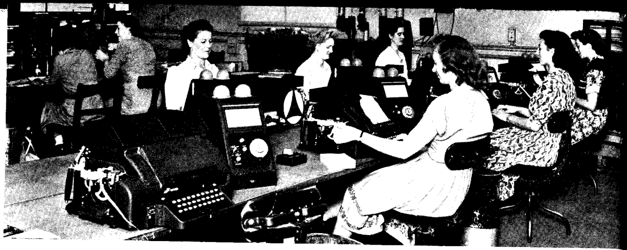
Suite of new teleprinter automatic switching positions in the Central Telegraph Office, London.
