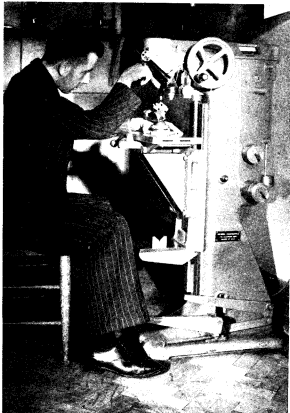
Fig. 4. The Diamond Pyramid Hardness Tester. A specimen under test.
