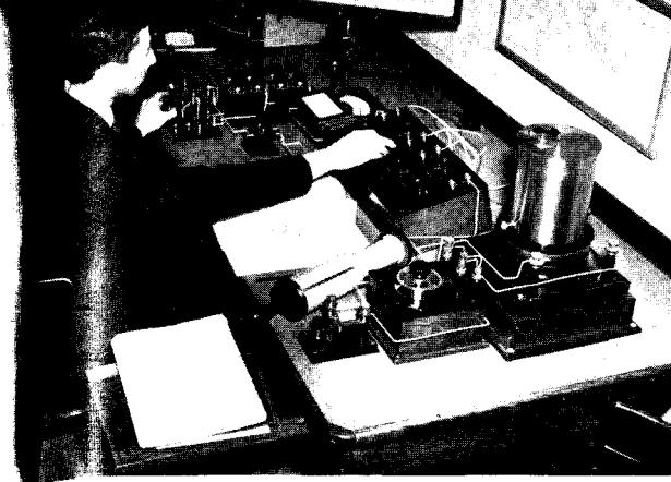
A student at the Cable & Wireless London Training School using a Wheatstone Bridge to determine the position of a fault in a long submarine cable
