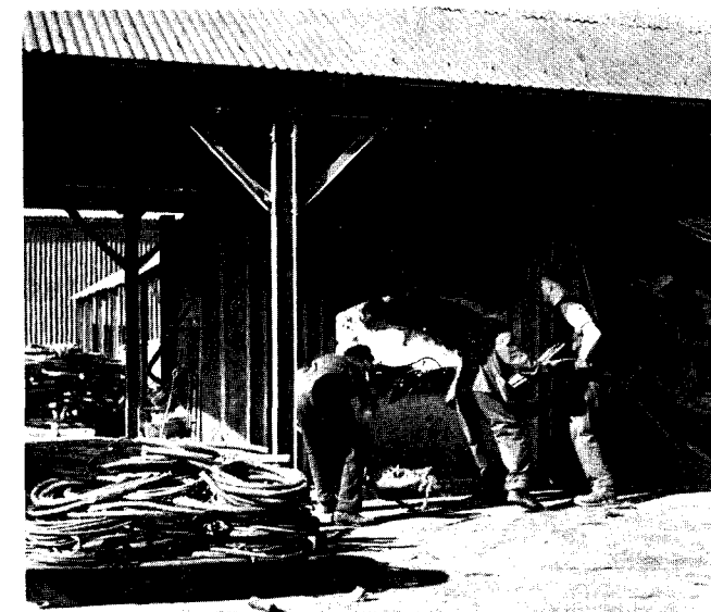
Feeding the melting pot with scrap cable
