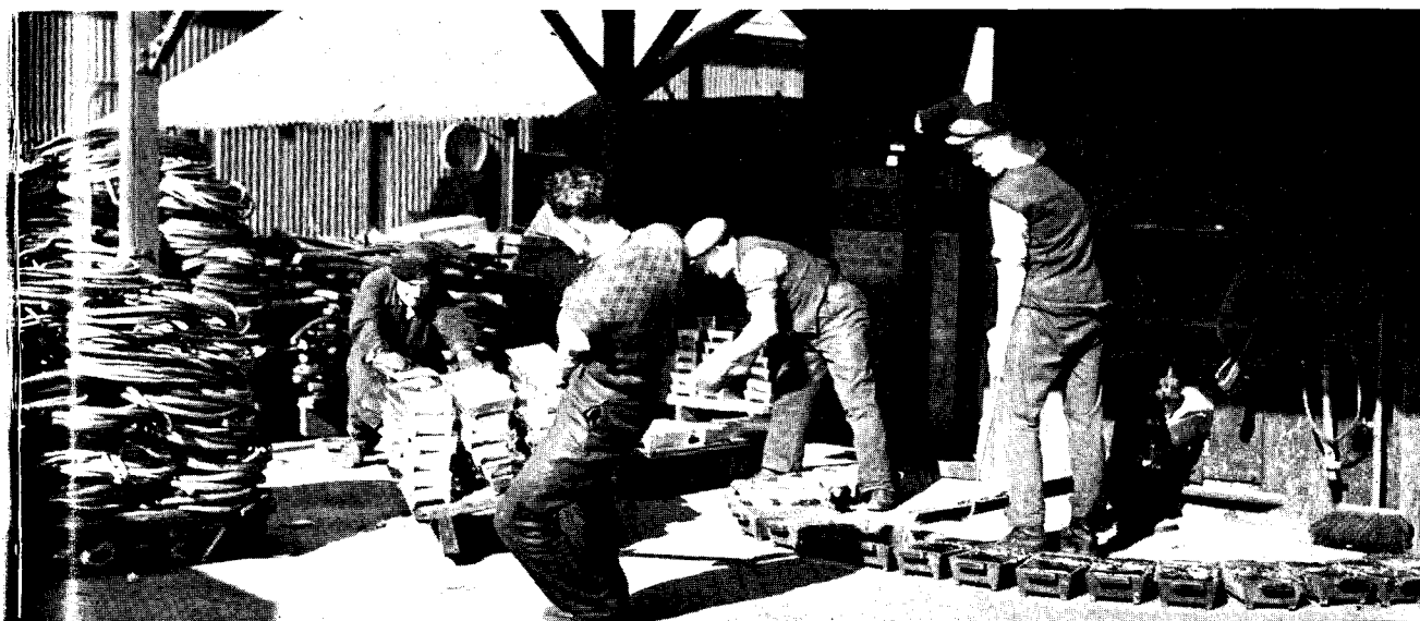
Running molten lead into ingots
