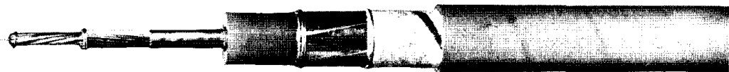
Lightweight cable with (l. to r.) central high tensile steel wire ; two layers of the same giving neutral strand ; single longitudinal copper tape outer conductor ; polythene insulation ; six aluminium tapes outer conductor ; cotton tape with common inhibitor; polythene protector sheath
