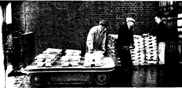
The old method of stacking lead ingots. Each ingot weighs from 60 to 80 lb.
