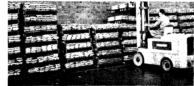
Pallet loads of ingots being stacked by a fork lift truck. Thirty-six ingots, weighing 2,160 lb., are handled in the time taken by one man to lift one ingot
