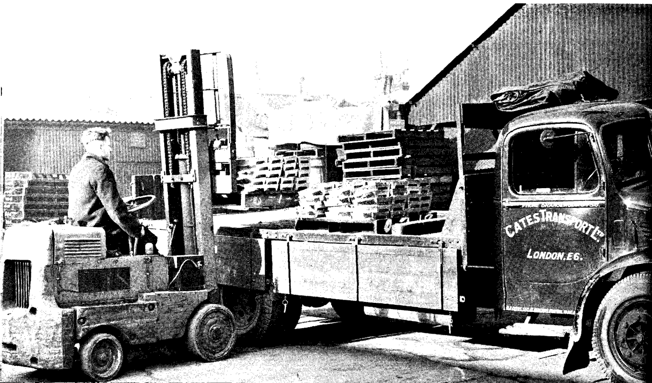
An open-sided lorry can be loaded to capacity with lead ingots by a fork truck in a matter of minutes
