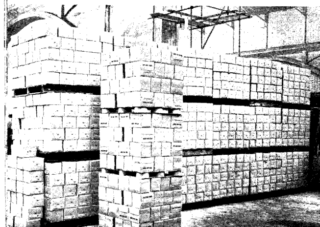
A typical stack of palletised telephones. Those in the foreground have been assembled on expendable cardboard pallets and bonded with special glue which does not injure the cartons when the load is broken down
