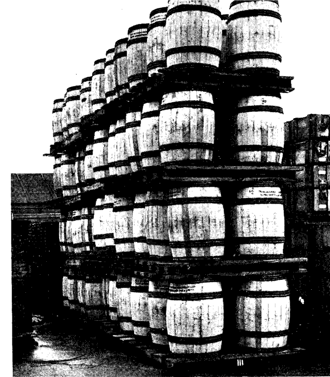
Barrels of insulators become easy to handle, four at a time, on a pallet. Headroom is used to advantage
