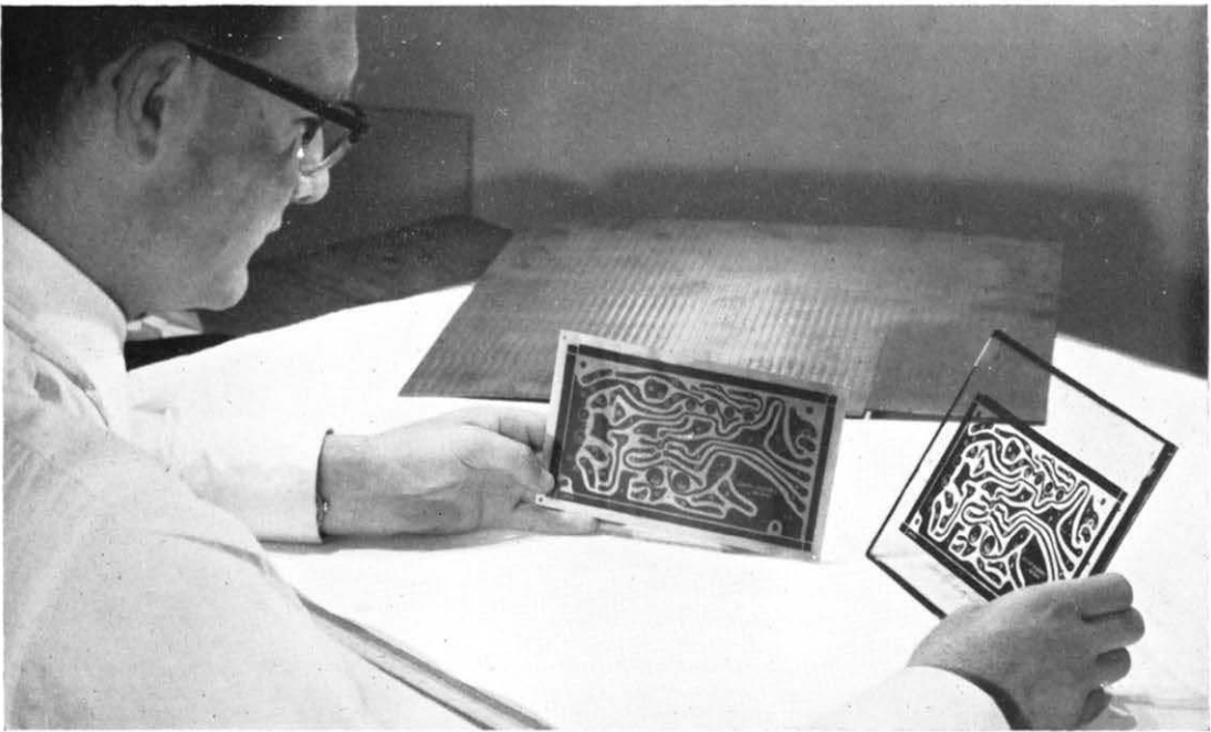
Fig. 5: Checking the developed image on the copper laminate against the negative
