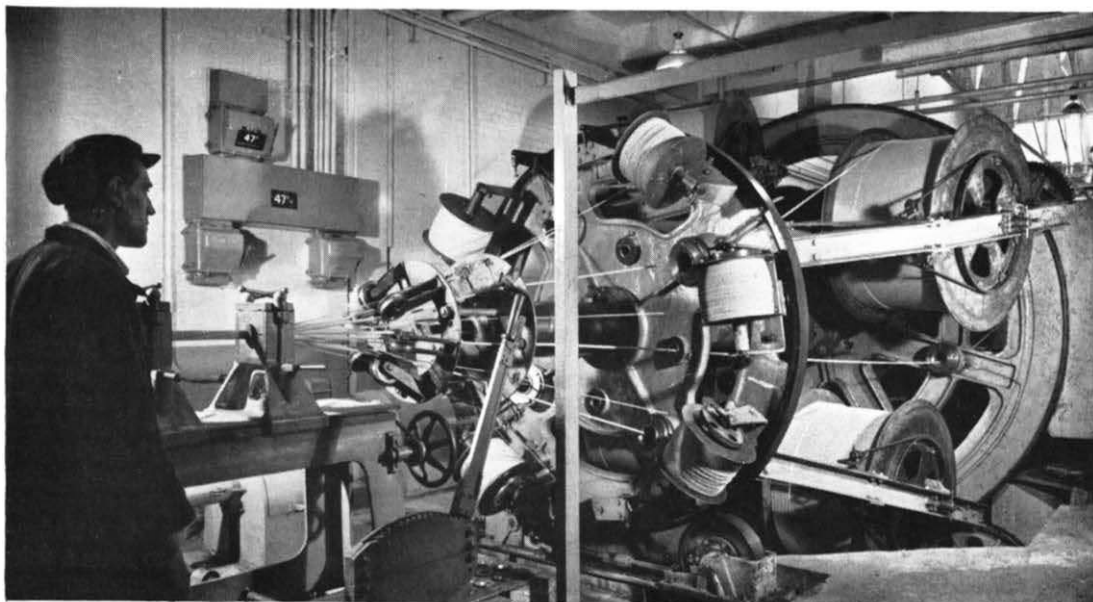
Stranding or laying-up— combining a number of conductors together
