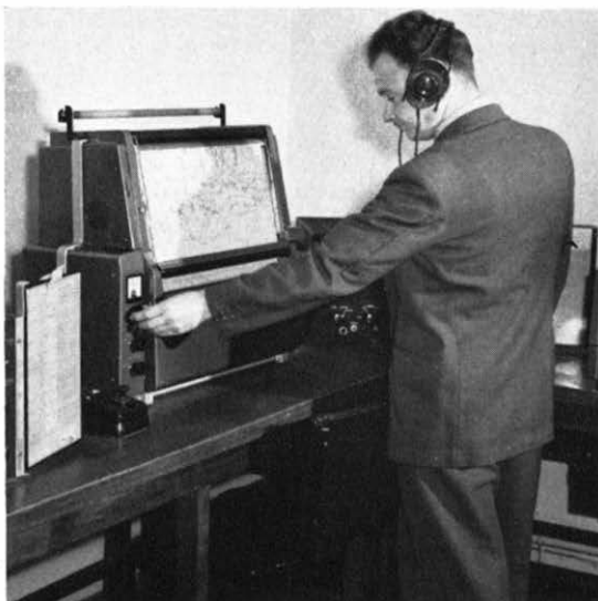
Facsimile Recorder. (Courtesy of Muirhead & Co. Ltd.)
