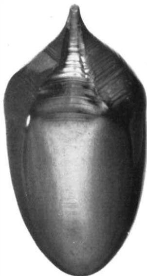
A crystal of germanium . . . "Crystal growing is the most delicate step of the whole process"
