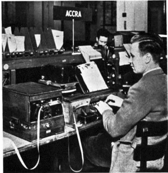
Transmission in the Main Instrument Room: operating the keyboard perforator into the transmitter
