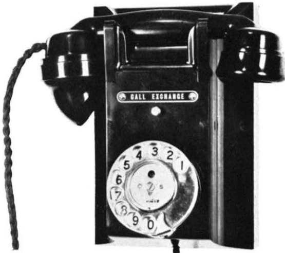
Fig. 4 : Interim type : this used as far as possible the same parts as the table telephones
