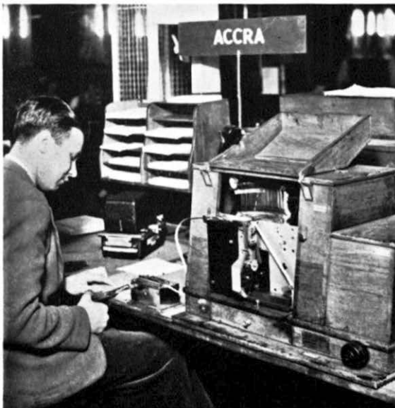
Reception in the Main Instrument Room: telegram being received on direct printer and gummed on a delivery form
