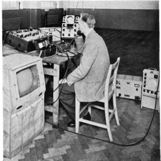
Fig. 4: Intermediate video repeater point at Cardiff automatic telephone exchange
