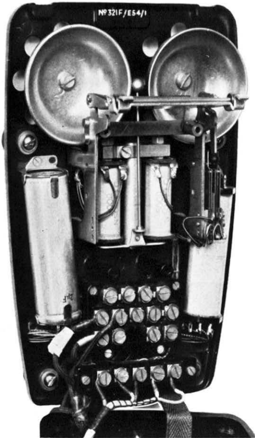
Fig. 2 : The principal parts are mounted on a die-cast base plate, the case being a plastic moulding fitting over the base
