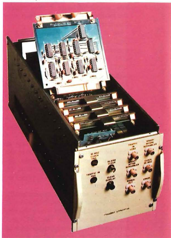
Transmit apparatus of a 120 Mbit/s line transmission system showing the new technique of cassette construction.
