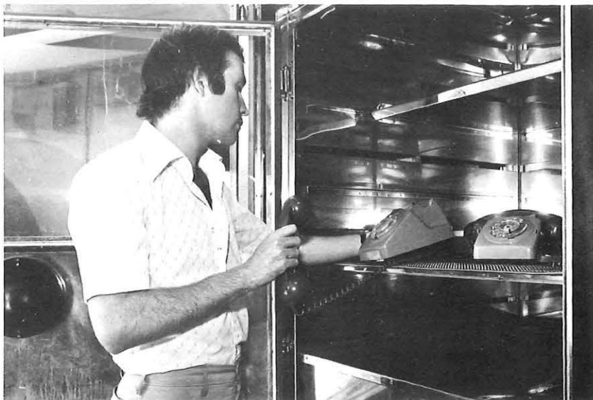
Tony Knight removes a batch of telephones which have undergone climatic storage tests.
