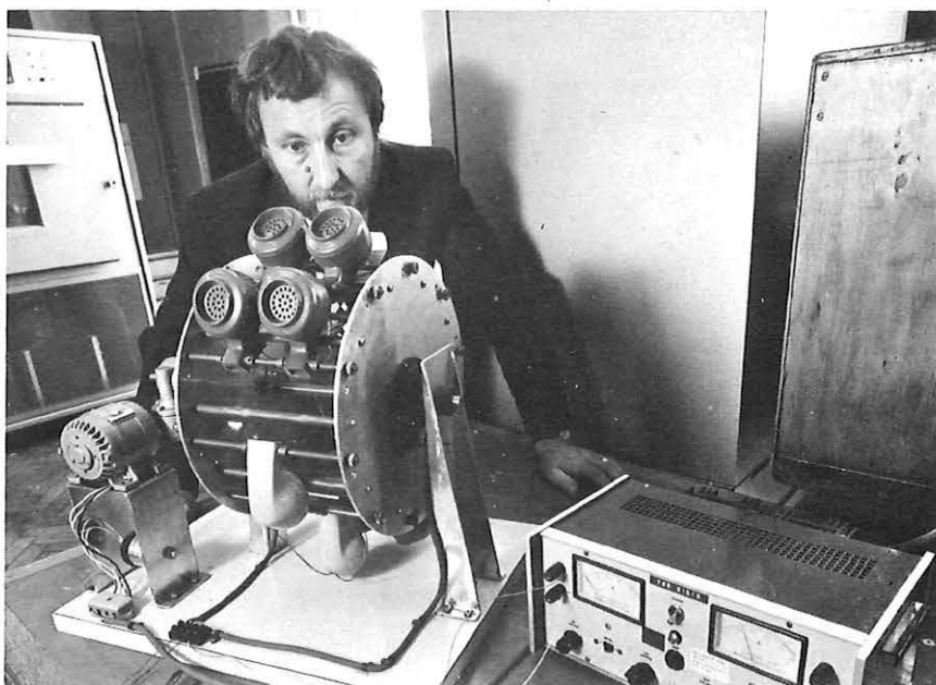
Assistant Executive Engineer Alan Hill keeps a close eye on telephone transmitters undergoing shock test treatment.
