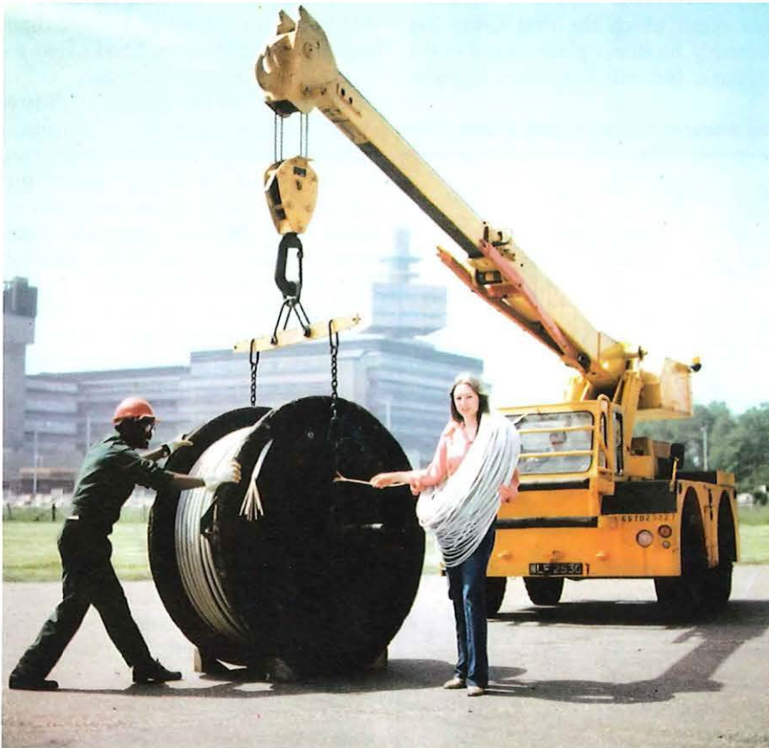
Technician Fred Walker and Louisa Hareduke a CA in the library at Martlesham show the difference in bulk between 500 metres of coaxial cable and the same length of optical fibre cable. Both can carry 16,000 telephone circuits but the coaxial cable on the drum weighs five tons while the optical fibre cable tips the scales at a mere 25lbs.
