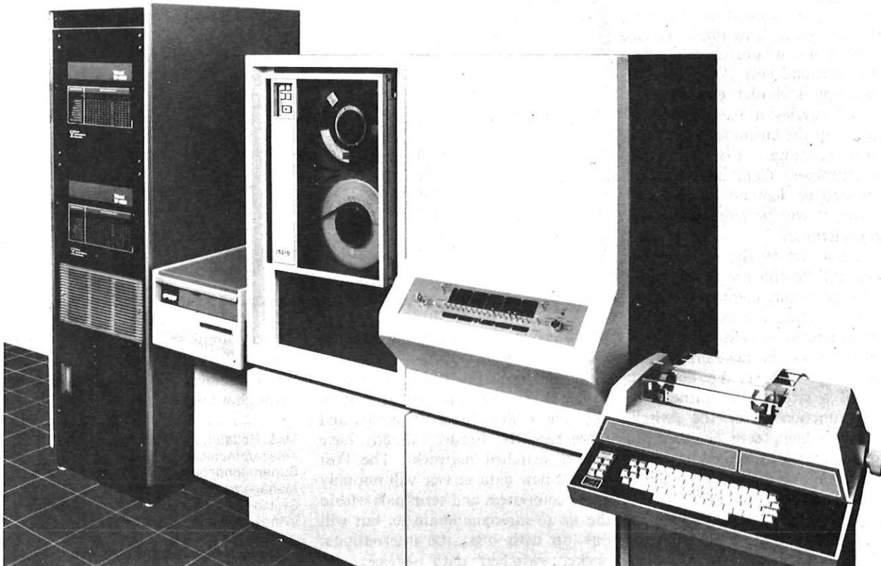
On the left is the TP4000, the basic switching equipment at each packet switching exchange. The rest of the equipment is used in London's Network Management Centre and can monitor continuously the performance of all the PSEs in the network.
