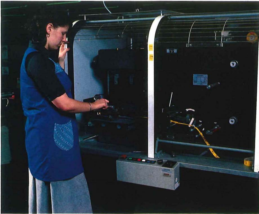
Assistant Factory Technician Julie Allaway changes the type face in a hot press printing machine.
