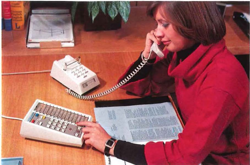
The TD Callmaker one of the new repertory diallers due for introduction throughout 1979.
