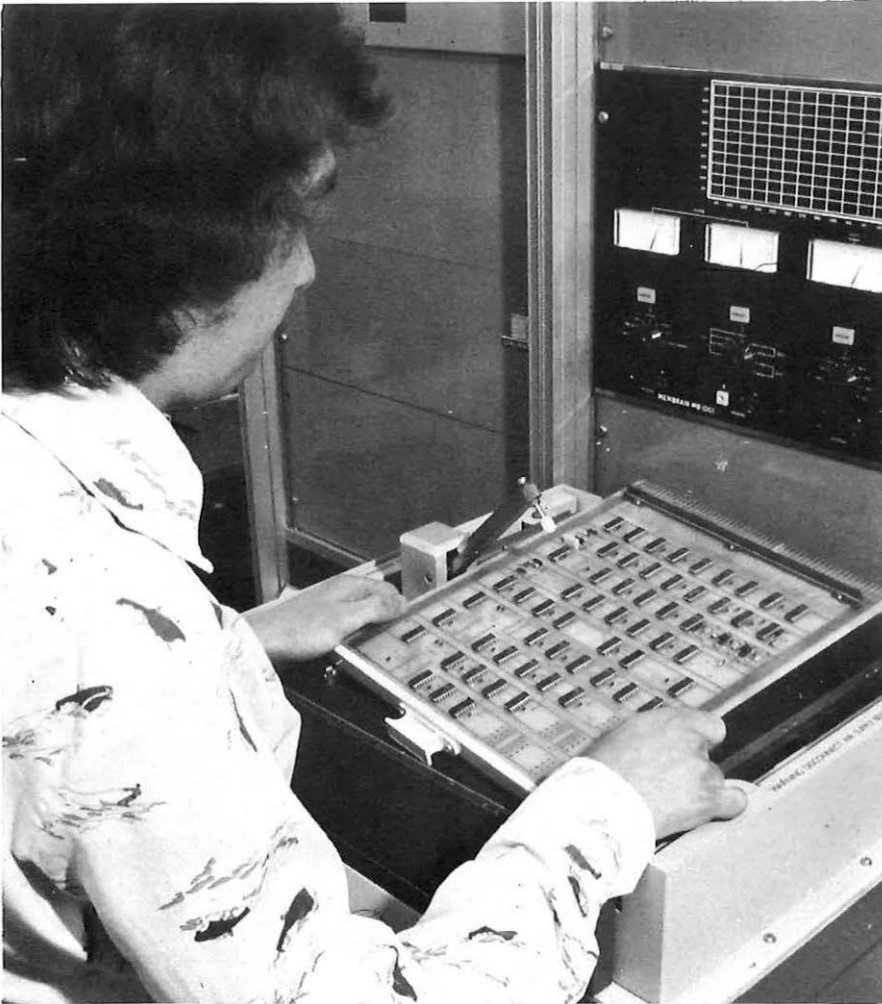
Automatic testing of System X boards takes place at STC's New Southgate factory.
