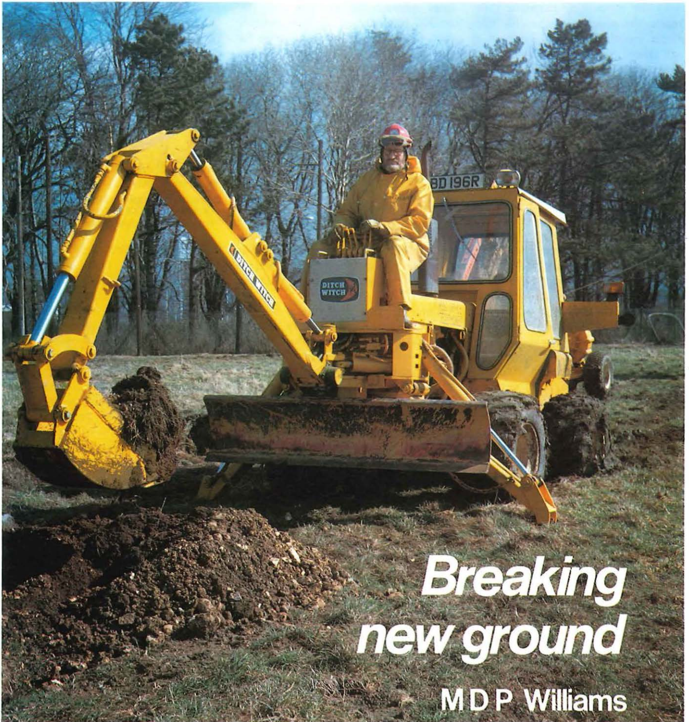
Instructor/Engineer Charles Baxter of Bletchley RTC demonstrates the backhoe type excavator at the front of the Ditchwitch.
