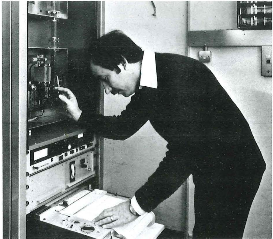
Executive Engineer Ray Bell calibrates one of the 12.1 GHz radiometers which are being used to measure 'sky noise'.
