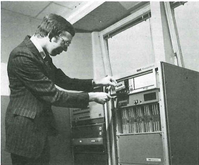
Executive Engineer Bob Brown of Telecommunications Development Department removes a cassette from the computer to obtain the monthly results from a MAC. These then undergo national analysis.
