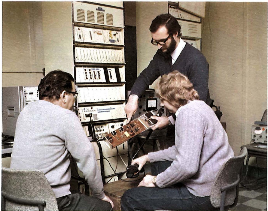
Jim Hudson, a lecturer at the Technical Training College, points out the power feed unit on a 24 channel pulse code modulation line system.
