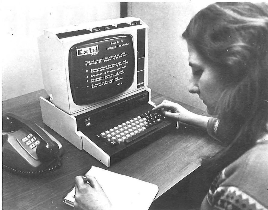
This desk top receiver for the business user has a special typewriter keyboard of particular benefit for the deaf enabling them to send messages and have them displayed in words on the screen.
