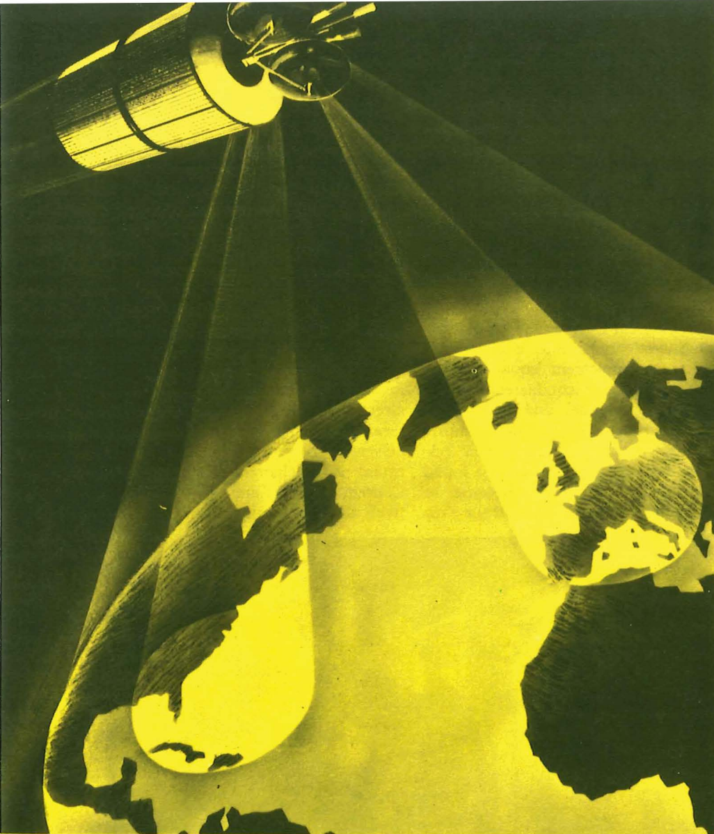
An artist's impression of the spot beam method of increasing satellite capacity.
