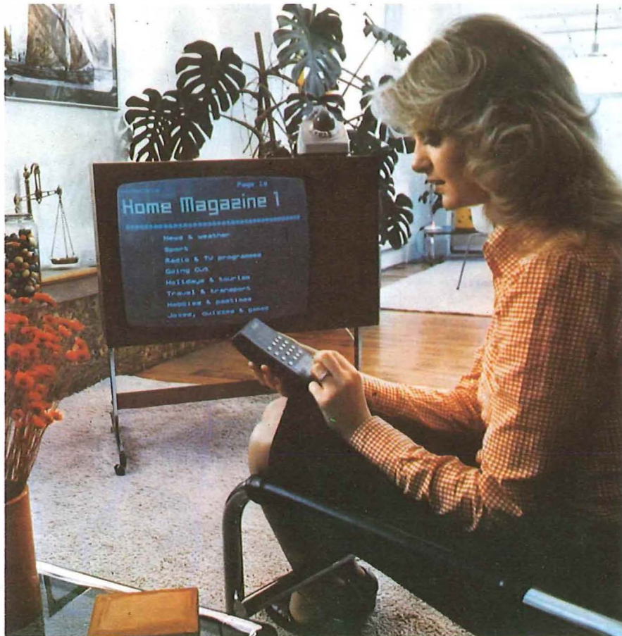
At home the Prestel user has a receiver with a small remote push button unit covering the numbers 0 to 9, enabling her to select the desired page of information.
