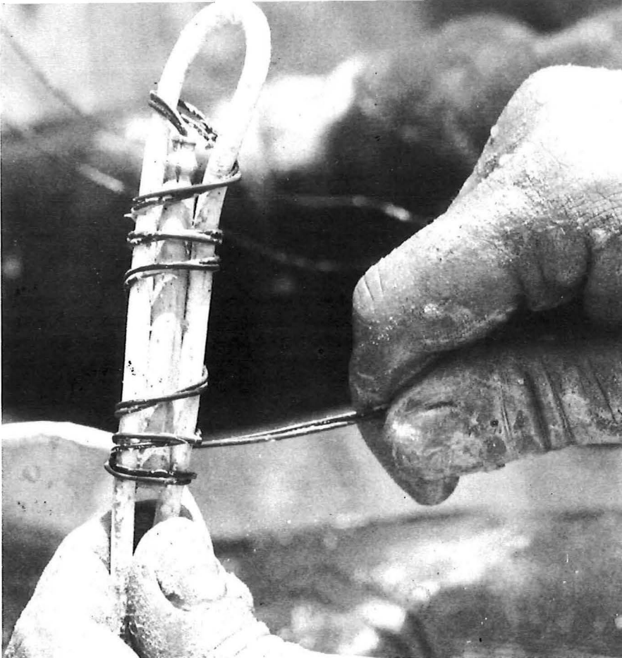
A cord is tied securely to the detonator before it is carefully placed in position.
