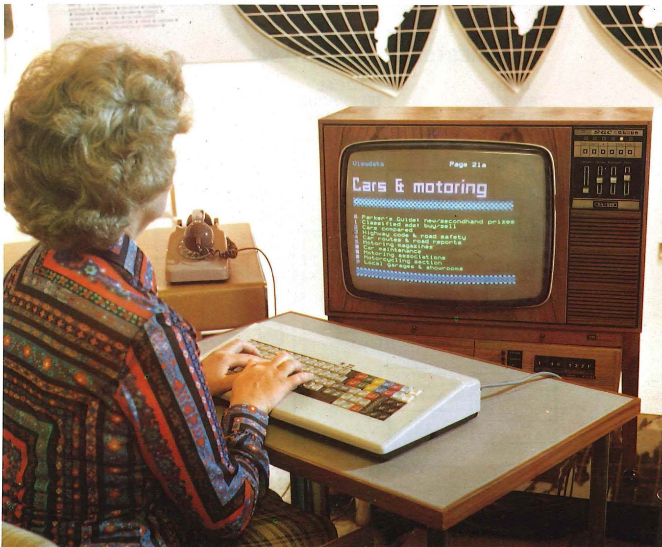
Firms supplying information to Prestel users can put their "pages" into the computer store by using a special control keyboard.
