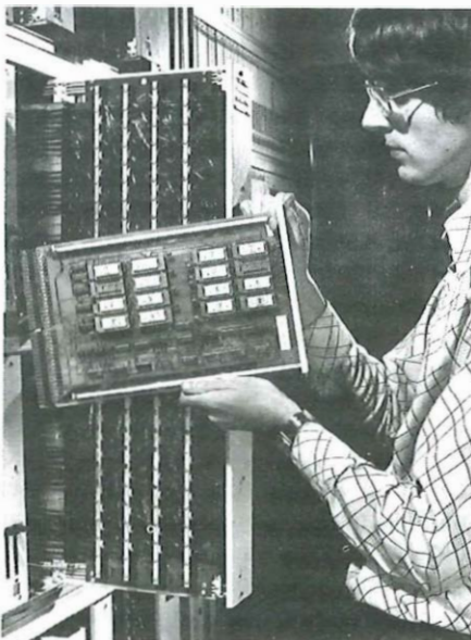
TXE4A's reprogrammable read only memory store shows the space saving when compared with the threaded wire equivalent of TXE4 in the background.
