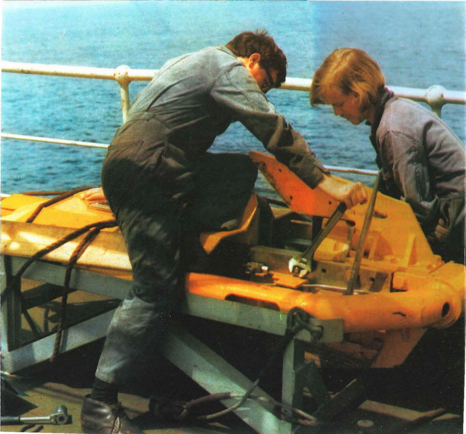
Final adjustments are made to the cutting grapnel (below) before it is lowered into the water during its sea trials.
