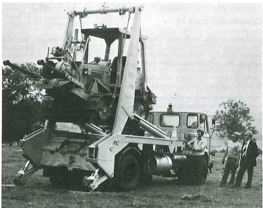
A purpose-built skip loader for carrying a mole plough tractor or other heavy engineering plant across difficult countryside, is put through its paces in Cardiff Telephone Area. The loader was designed and built by Powell Dyffryn to specifications laid down by Mr Bernard Wood, head of the Motor Transport Group at Wales and the Marches Telecommunications Board Headquarters.
