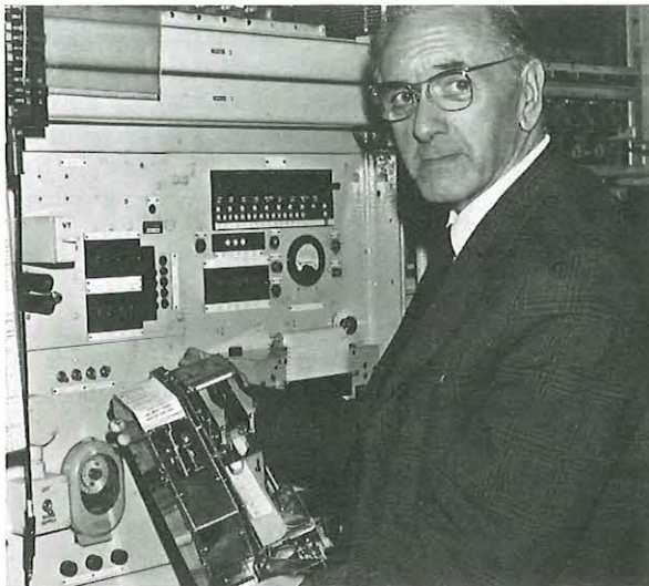
Technical Officer Bob Brace – £150 for designing an outrigger which enables a printed circuit board to be pulled out of the main apparatus rack during exchange maintenance.
