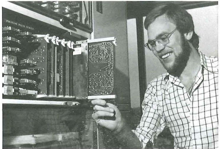
Technical Officer Bob Brace – £150 for designing an outrigger which enables a printed circuit board to be pulled out of the main apparatus rack during exchange maintenance.
