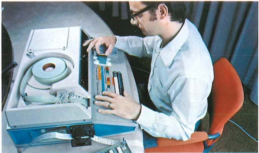
A microwave memory chip is reprogrammed by Technical Officer Mike Bloomfield from the paper tape master record.
