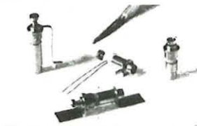
MINIATURE UHF TRIMMER CAPACITORS TYPE PTUTUT: This range of trimmers was first developed for the UK III satellite. The ability of the capacitors to operate over a wide frequency range enables them to be used even into the microwave region with complete confidence. (Actual self resonance frequency at C max type PTU1.2 is 4GHz). Capacitance range 0.2pF to 3pF. Printed circuit chassis, and strip line styles available.
