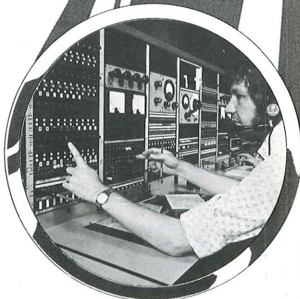
Using the facilities of a test desk at Cambridge Trunk Maintenance Control Centre, Technical Officer Maurice Flinders localises a fault on a circuit.
