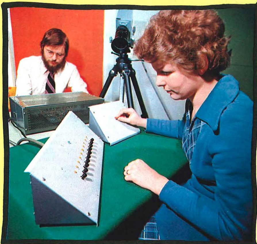
At the special outstation now being set up in Ipswich, Executive Engineer Martin Cooper records on videotape user response to light emitting diodes which are being introduced on various items of customers' equipment in place of filament bulbs.
