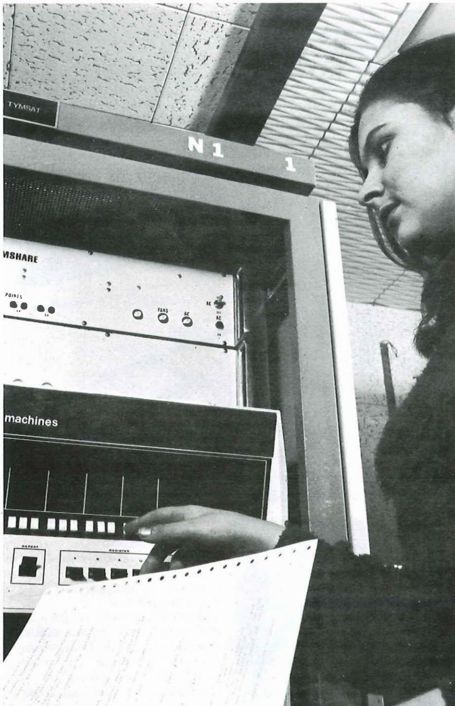
The data concentrator at Tymcom's office in West London is set to enable the Post Office to gain access to the TYMNET network.
