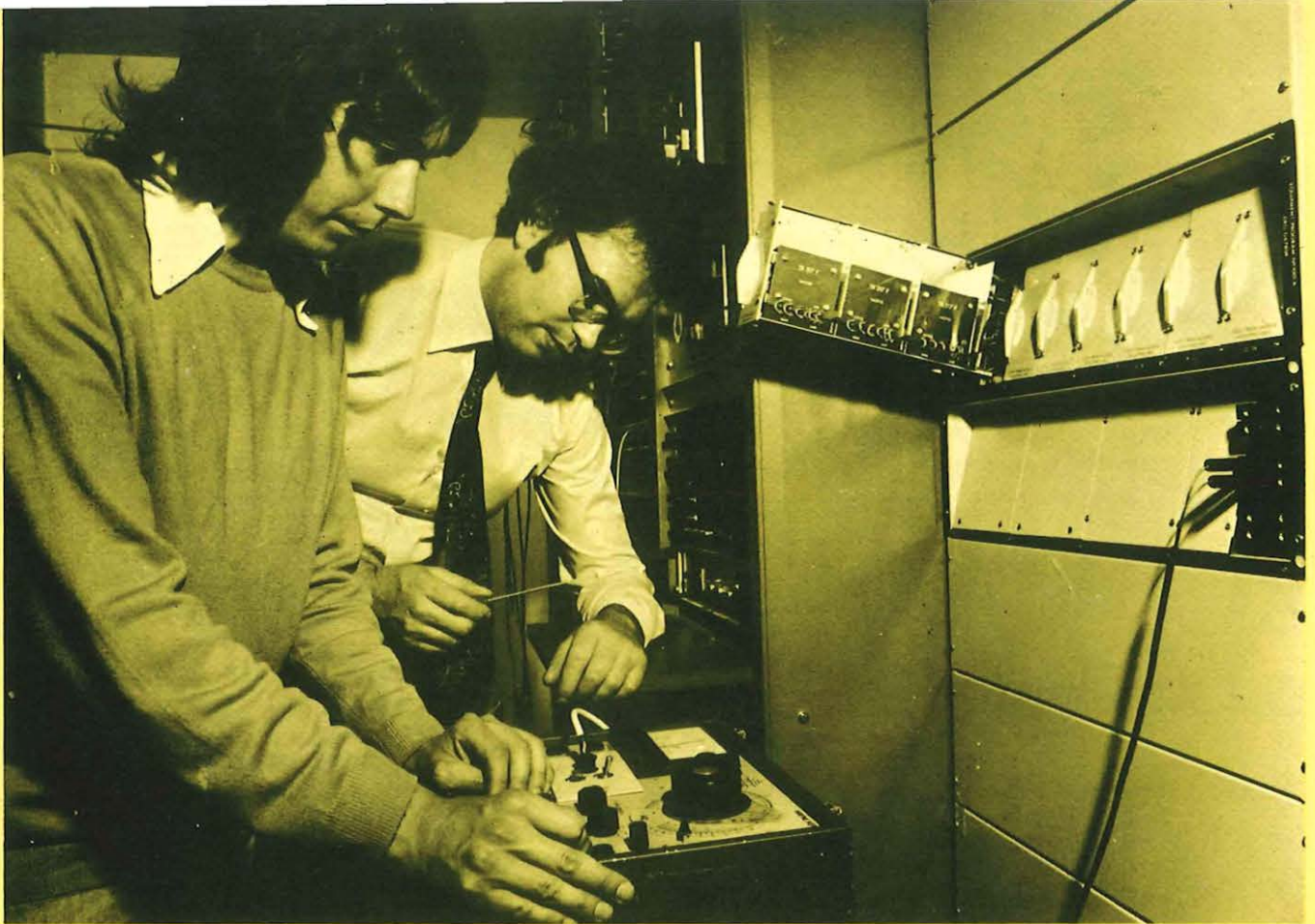
Post Office Technical Officer Chris Brooks, left, watched by Radio Orwell's chief engineer Richard Allison, tests the overall performance of the private circuit which links the Ipswich studios with Independent Radio News.
