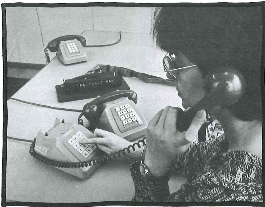
A volunteer tests "button action" on various types of keyphone to compare the feel and touch with standard equipment.
