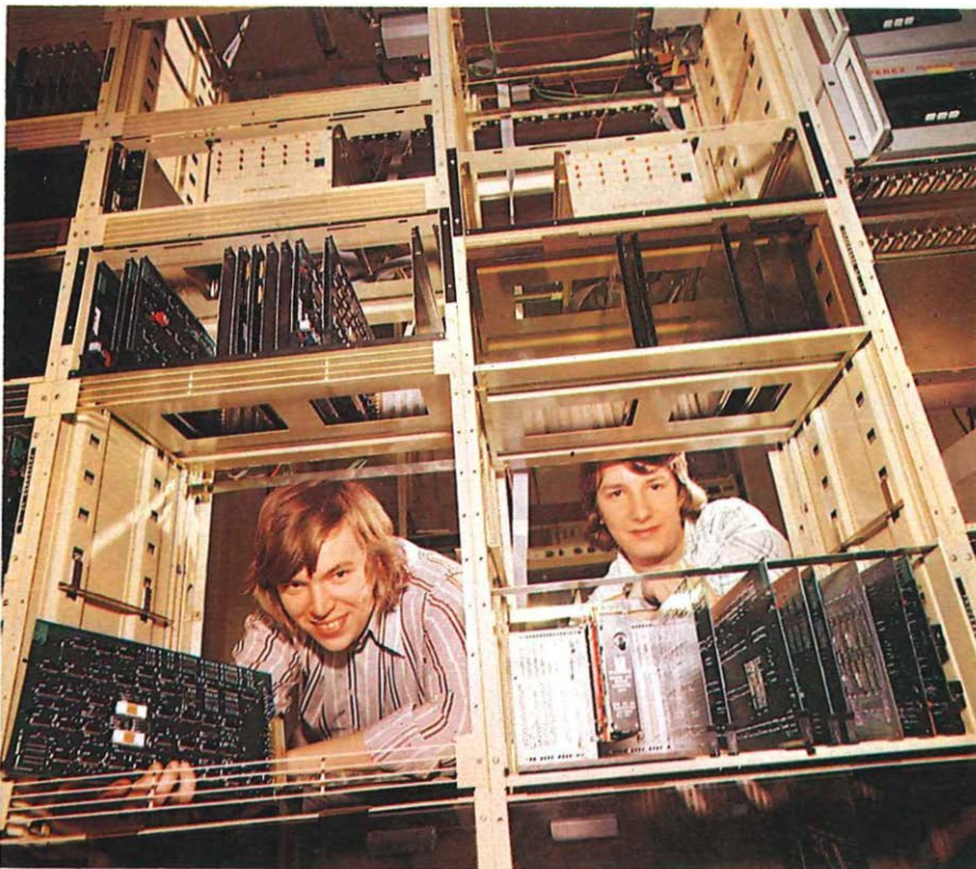
A working laboratory model of the processors for automatic call recording equipment (ACRE), the design of which uses modern computer techniques to simplify call handling for operators. A number of patents are involved in its development, and seen here are Technical Officer Alan Farmer, left, and Technician Dave Windsor who were responsible for certain elements of the circuit design.
