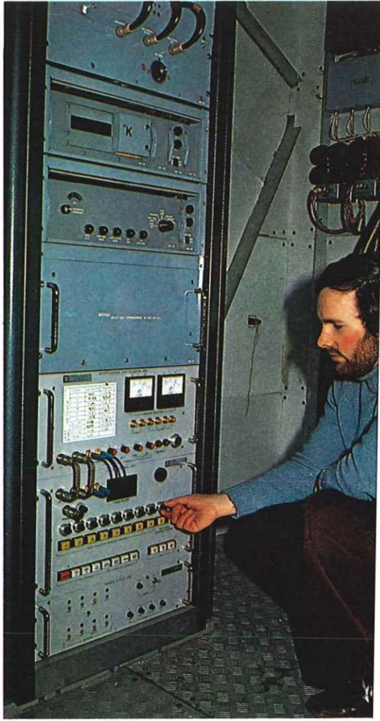
Mr Terry Pascoe, a Technician at Goonhilly, adjusts the frequency of the cancellation unit housed in the equipment cabin which is situated at the rear of the Aerial 1 reflector structure.
