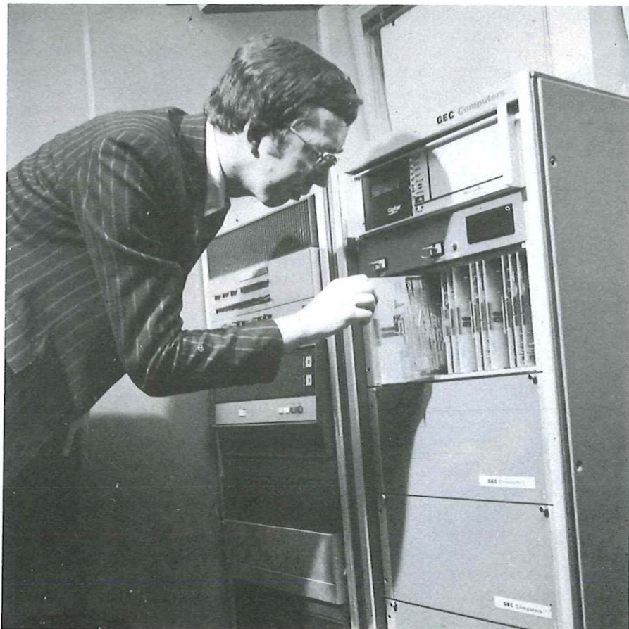
Mr Bob Brown, an Executive Engineer on the MAC project, inspects a sender/receiver which forms the interface between the MAC equipment and the Post Office test circuits.
