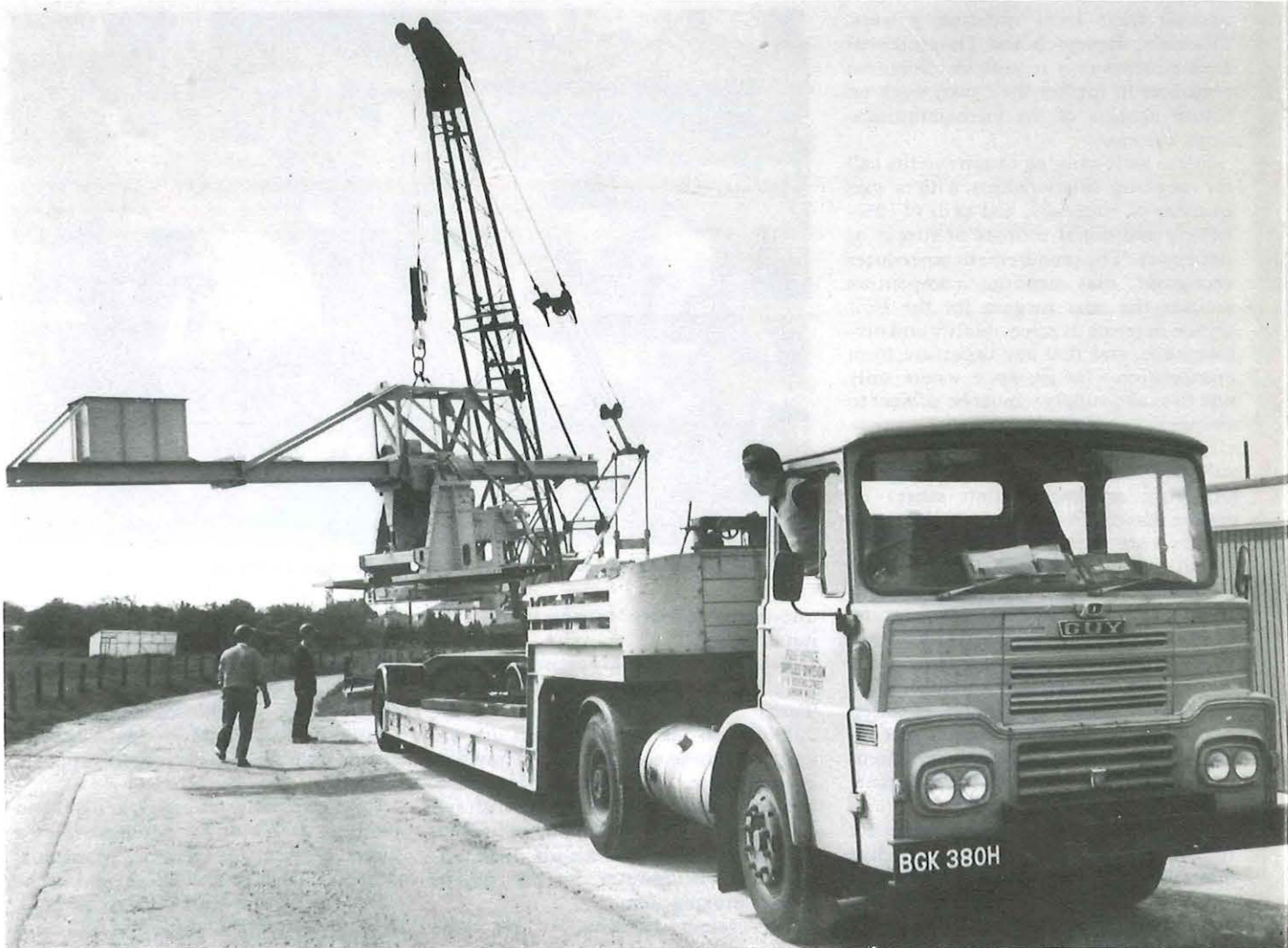
A Supplies Division vehicle prepares to transport a former naval gun mounting from Smallford in Hertfordshire to Goonhilly earth station for use in supporting a dish aerial.
