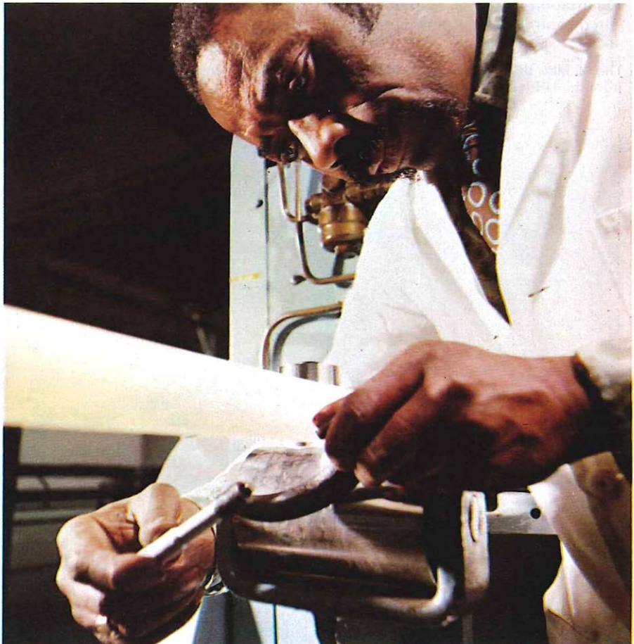
Below: During production of a submarine cable, its diameter is measured with a micrometer.
