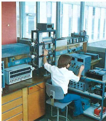
Lasers undergo life testing to measure their reliability for optical fibre transmission.
