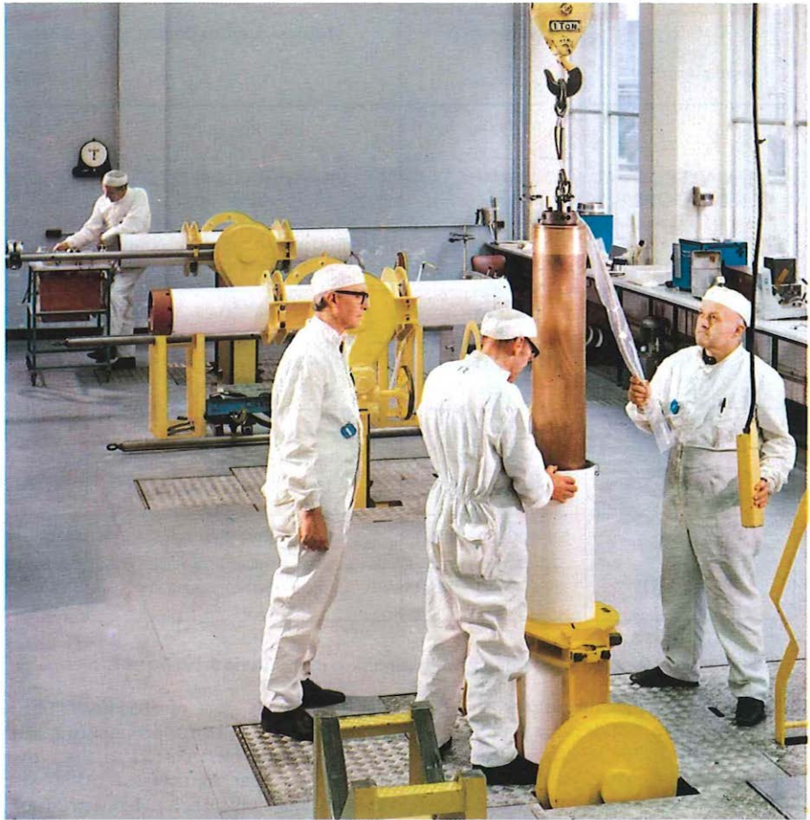
Above: A submarine repeater undergoes final assembly in the clean room facility at an STC factory.
