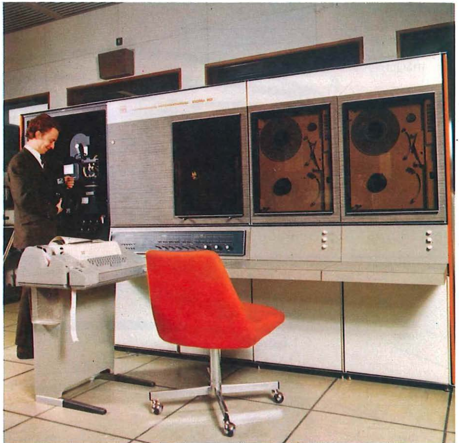
Above: The COMP 80 equipment at the Post Office's Leeds computer centre, which processes telephone directory information and outputs it on microfilm in a form suitable to print updated records for Directory Enquiry operators.
