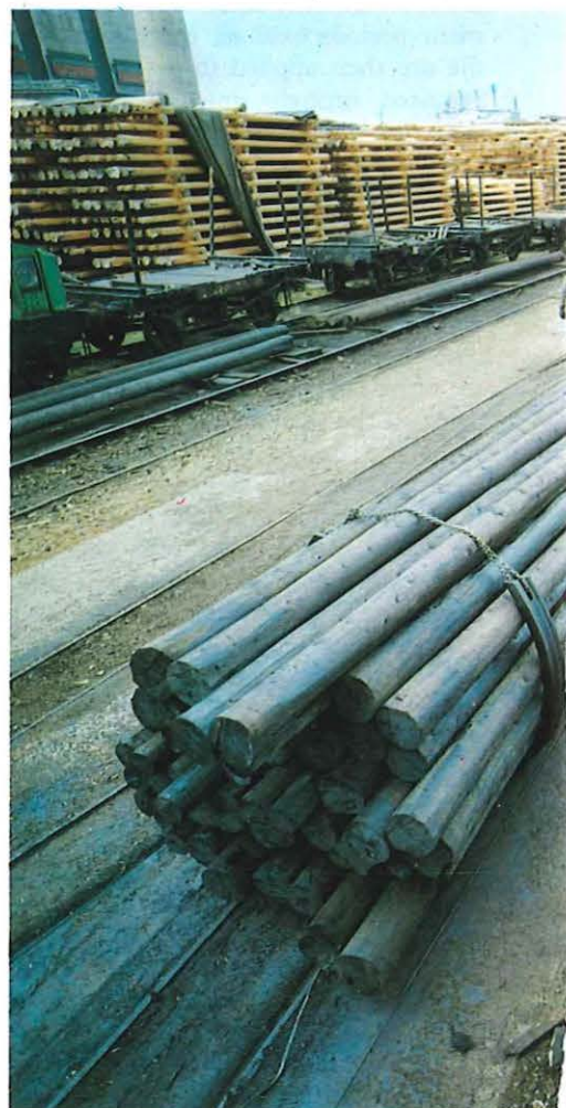
Below: Trolley loads of wooden poles emerge from the creosot tank, about 165 poles at a time.
